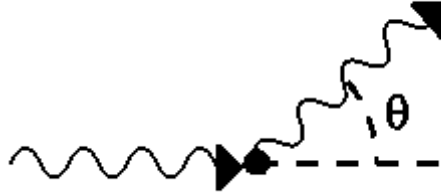
Figure 3.4 - Diagram of a photon coming in from the left and being scattered off an electron by an angle of \theta .
