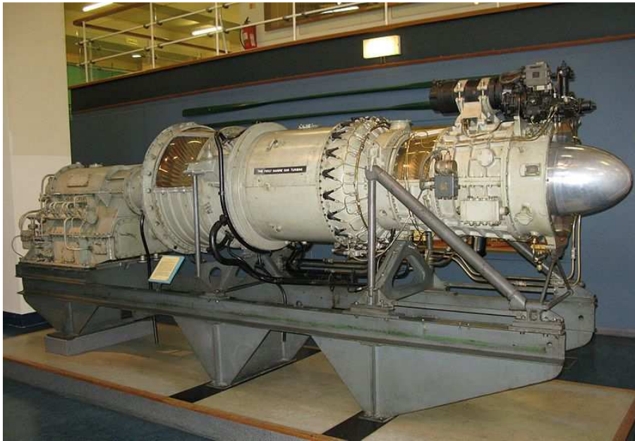
Figure 4 – Gatric unit preserved in the Science Museum London. The power turbine and gearbox are on the left. 30
