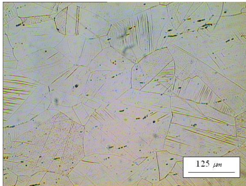
Fig. 5.2. Microstructure of the “as received” material, XZ section (longitudinal direction).
