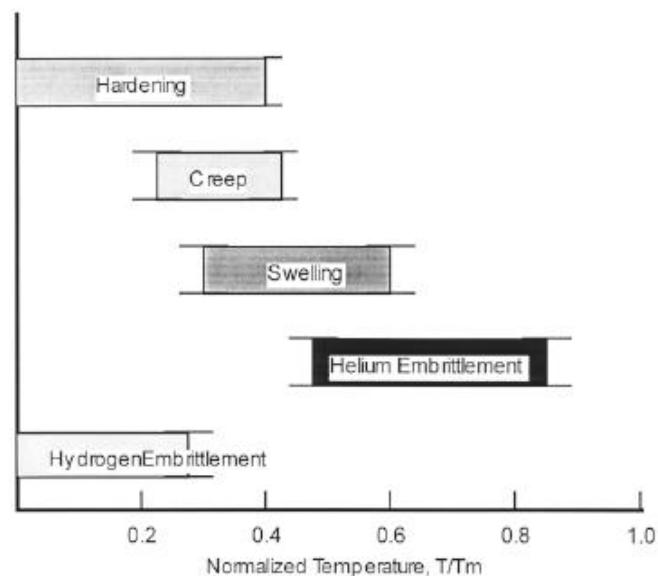
Fig. 2.24. Temperature ranges for the various types of radiation damage typical of radiated metals and alloys [82].
