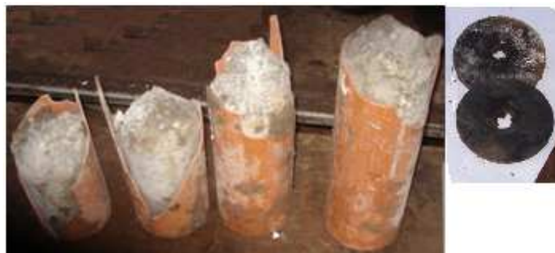
Figure 6-8 The penetrated tested witness concrete targets and the steel discs.
