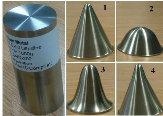
Figure 7-8 The zirconium solid cylinder (left) and the manufactured liners; 1: conical; 2: hemispherical; 3: bell and 4: bi-conical shape.
