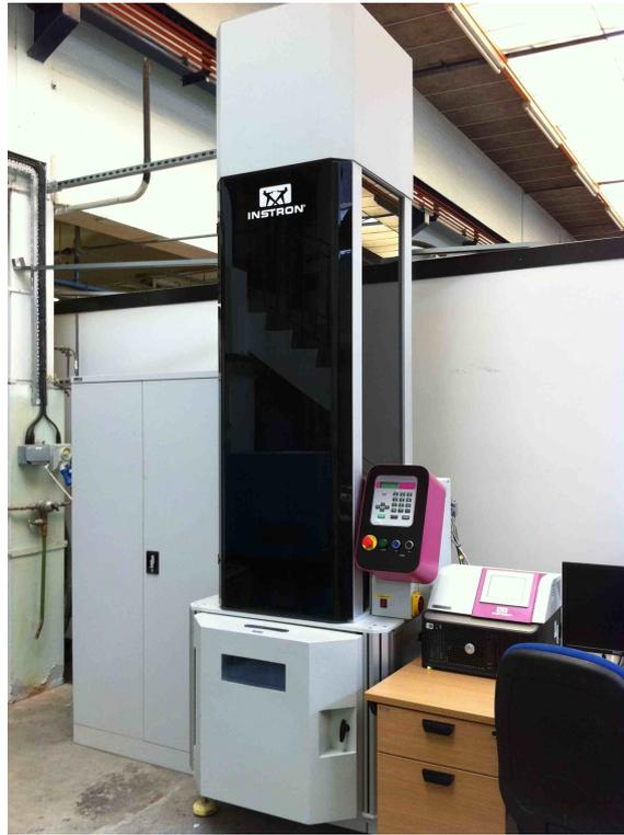
Figure 5.1: Instron CEAST 9350 drop weight impact testing machine.
