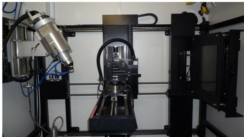
Figure 4.2: Nikon Metrology Custom CT bay with 225kV X-ray source (left), 5-axis sample manipulator stage (centre) and 2000 x 2000 pixel flat panel detector (right).
