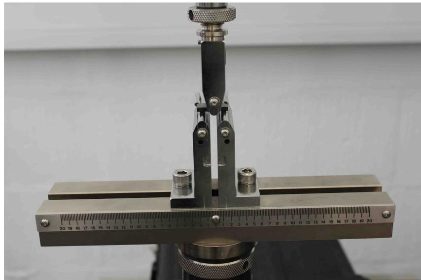
Figure 5.17: Interlaminar shear strength test rig with a sample in place
