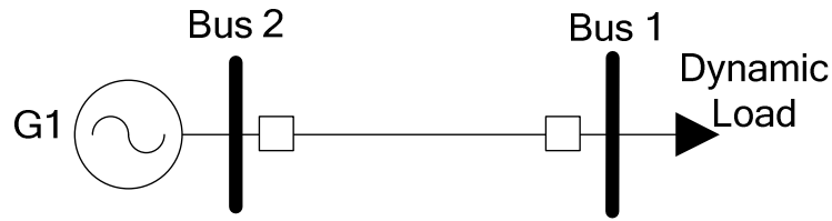
Figure 4-10: Single-line diagram of the two-bus system
