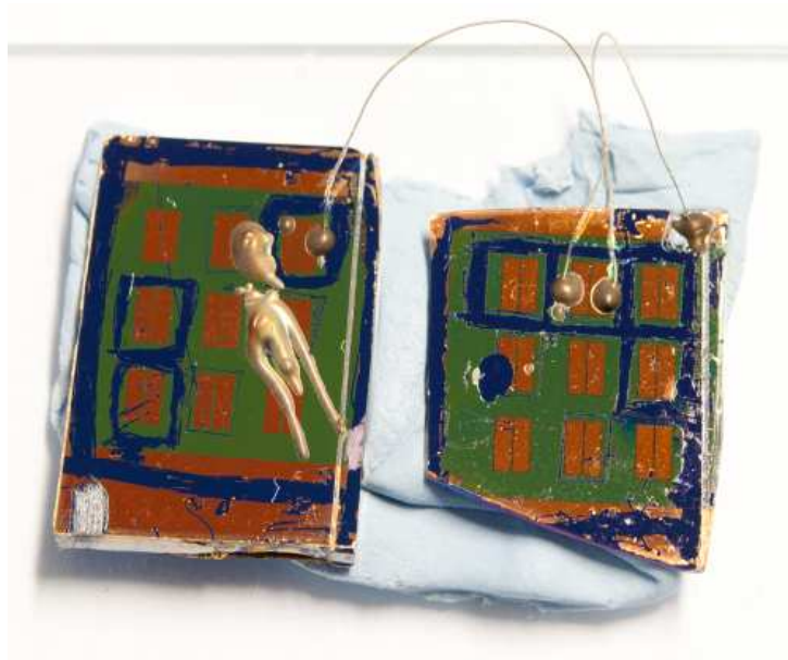
Figure_Apx F.7: The first functional organic inverter in UoM EEE fabricated on Si-SiO 2 substrates. PTAA is used as the active layer and (conductive) epoxy bonded wires were employed for forming interconnects.
