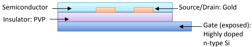
Figure 4.1: Structure of the single transistor.
