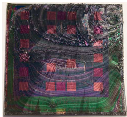
Figure_Apx F.5: Inverter circuit using PVP and drop casted TIPS-pentacene on Si-SiO 2 substrates.
