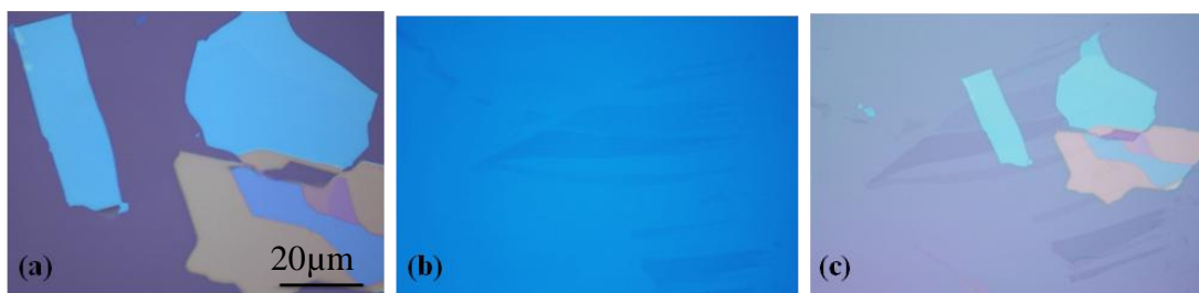
Figure 6.4: Sample fabrication for GBN hetero-structures. (a) light blue hBN flakes are \sim 30\text{ nm} thick (b) Graphene mechanically cleaved on PMGI-PMMA pre coated on Si/SiO 2 (c) Graphene flakes transferred on hBN flake.
