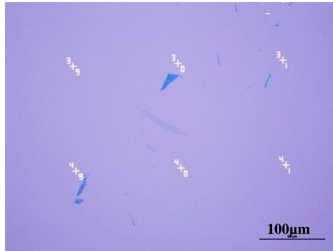
Figure 3.7: White light optical image of the micromechanically cleaved graphene on Si/SiO 2 substrate with alignment crosses patterned by mask aligner Karl Suss MJB3.
