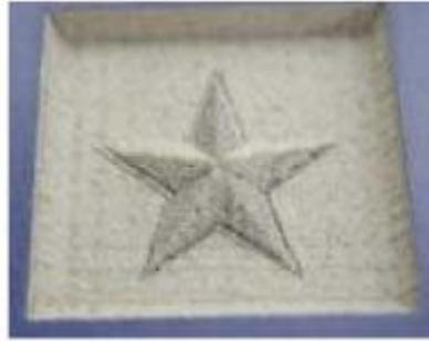
Figure 2.41 3D laser machining of a star shape in alumina ceramic [108]
