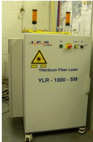
Figure 3.1 The IPG YLP-1000-SM fibre laser system
