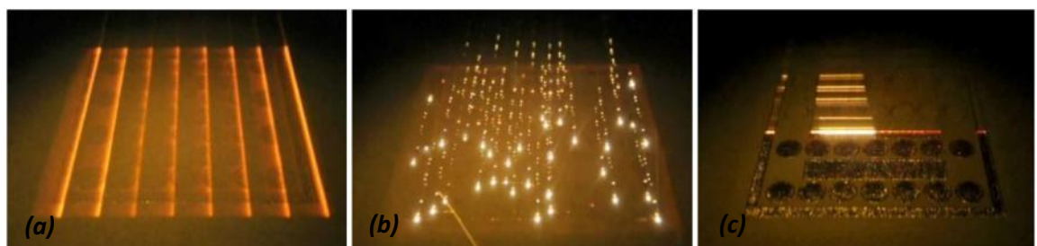
Figure 3.4: Photographs of the key processing steps in EBM; (a) powder preheating, (b) melting of component perimeter (contour) using a multi-beam mode and (c) hatching [92].
