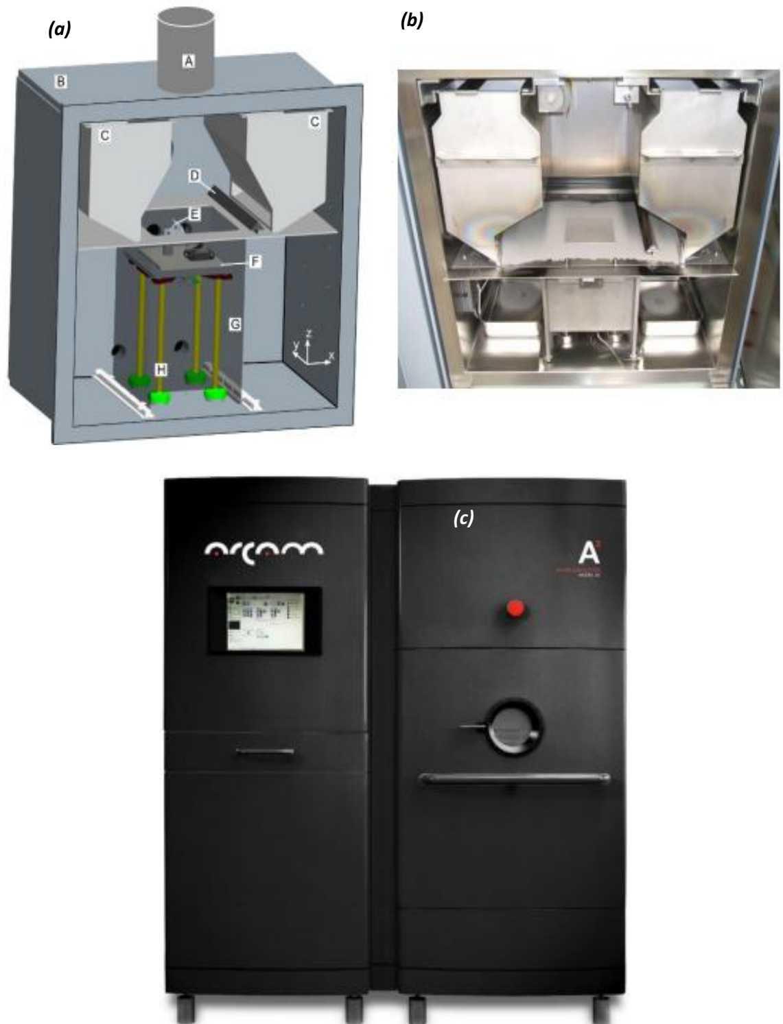
Figure 3.2: (a) Key components of the Arcam S12 e-beam AM machine, and control system; electron gun column (A), build chamber (B), powder hoppers (C), rake arm (D), component (E), base plate (F), build chamber (G), z-axis assembly (H), (b) photograph of the EBM build chamber and, (c) exterior of the Arcam S2 EBM machine [23, 112].
