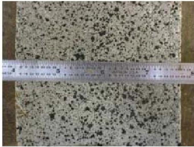
Figure 2-22: Shows the white and black spray paint for the large deformation; large viewed area and the feature sizes are measured [67].
