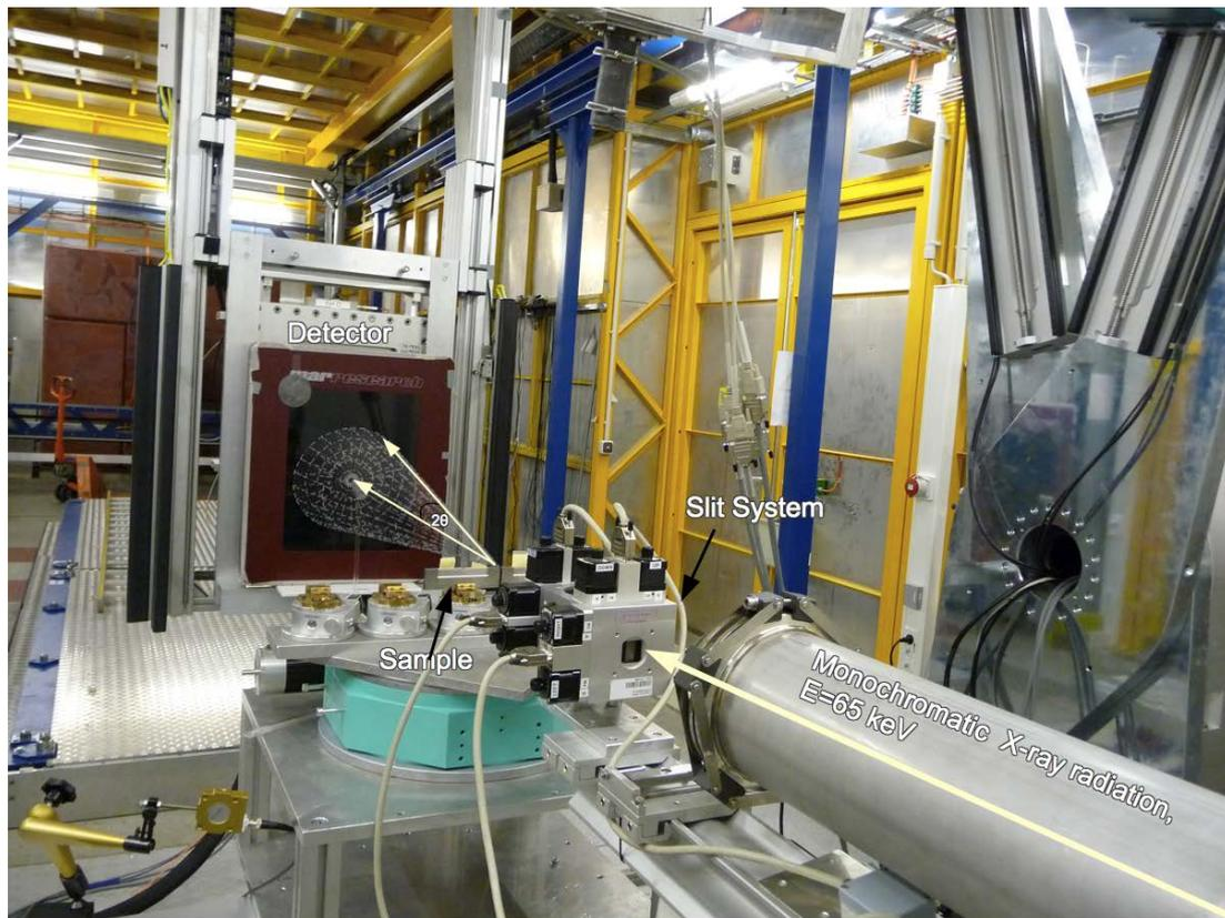
**Figure 3.9:** Experimental setup for thorough thickness transmission strain scanning of simulated leading edge Ti-6Al-4V sample on HARWI II beamline.
