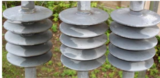
Figure 5.27 Drying differences between darker and lighter areas, the lighter side dried first
