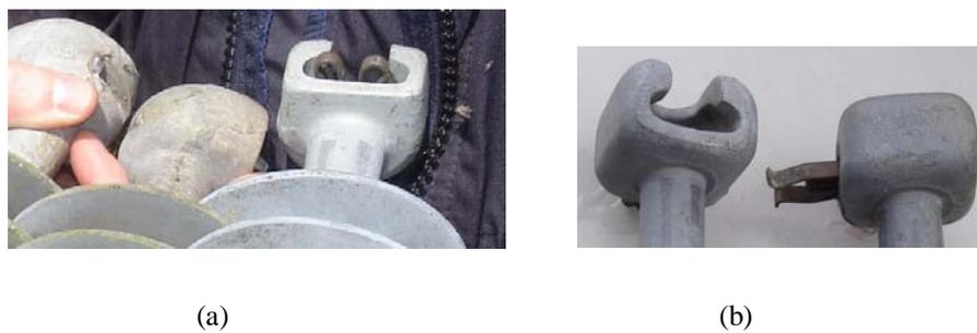
Figure 5.43 Differences between end-fittings (a) Circuit IV; (b) Circuit I
