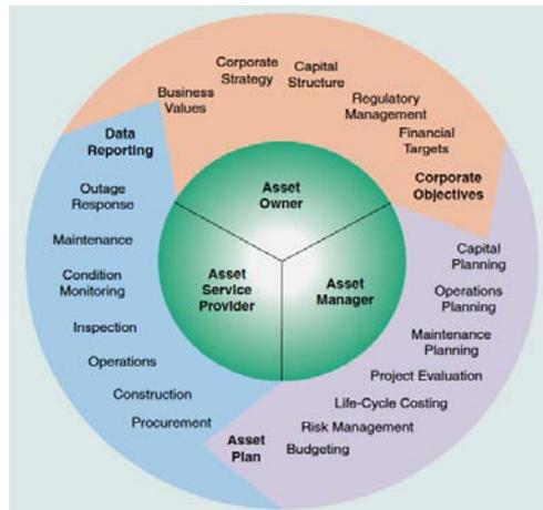
Figure 2.6 Asset management is based on three functions (asset owner, asset manager and asset service provider), a single process, and many decisions [4, 15]
