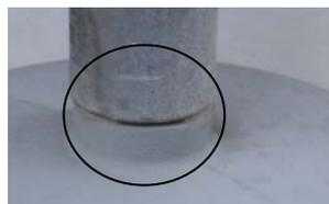
Figure 5.24 Void in the interface polymer/socket end fitting
