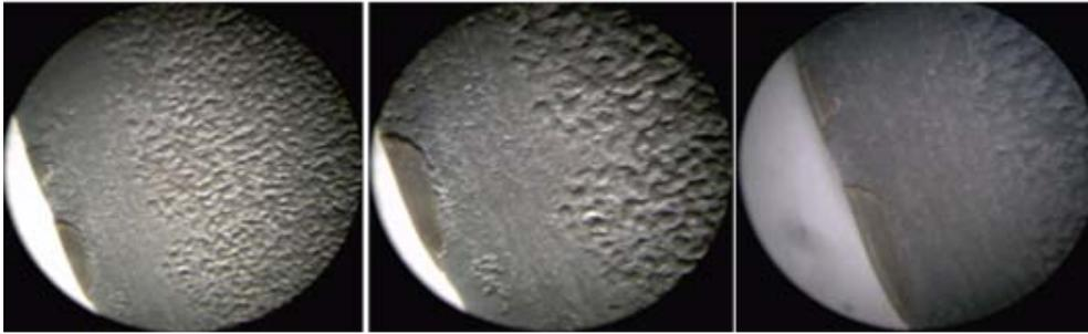
Figure 5.38 Local pollution in one of the sheds. Contaminant deposition detail, a less polluted ring is surrounding the rim of the sheds
