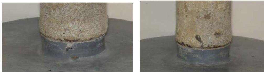
Figure 5.37 Severe erosion is detected in the interface polymer/end-fitting seals
