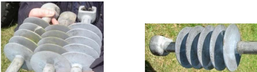
Figure 5.39 Organic pollution deposition; (a) green biofilm layers and bird droppings, (b) darker spots
