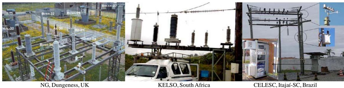
Figure 3.17 Test Stations of Insulators [101-104]
