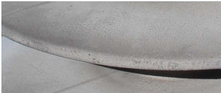
Figure 5.28 High roughness on the surface of an insulator
