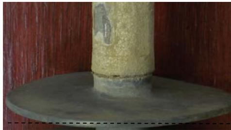
Figure 5.36 Undulations detected in some sheds close to the South side terminal; high level of corrosion on metal end-fittings
