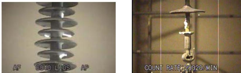
Figure 3.5 Corona discharges detected on polymer insulators using IR and UV integration [60]
