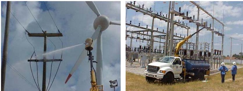
Figure 3.20 Robot developed to wash insulators. View of the truck and patrol members [110]
