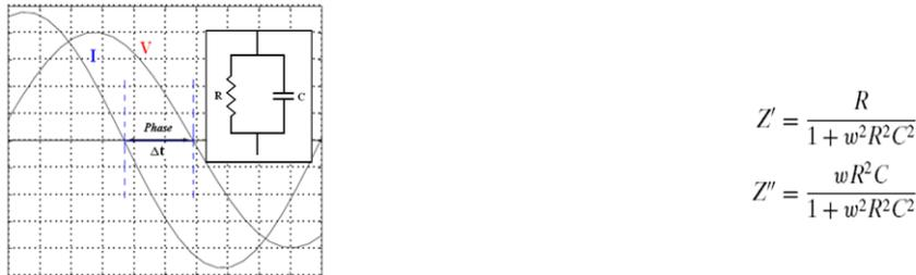
Figure 5.46 Impedance or admittance estimation
