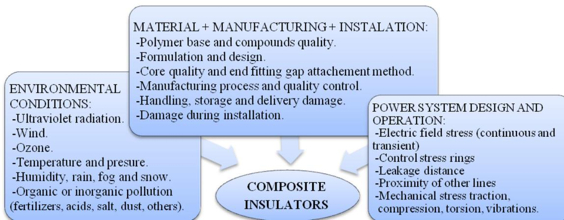
Figure 4.1 Main factors influencing composite insulators performance
