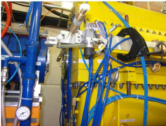
(a) Motor and pulleys secured to the IHS.
