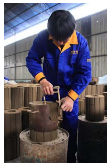
Figure 4.7 Cutting the opening in a clay combustion chamber, Shengzhou Stove Manufacturer, China. Photo: Martin Wright/Ashden Awards for Sustainable Energy
