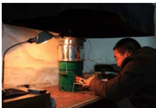
Figure 4.8 Emissions testing. Loading wood into a stove, Shengzhou Stove Manufacturer, China. Photo: Martin Wright/Ashden Awards for Sustainable Energy.
