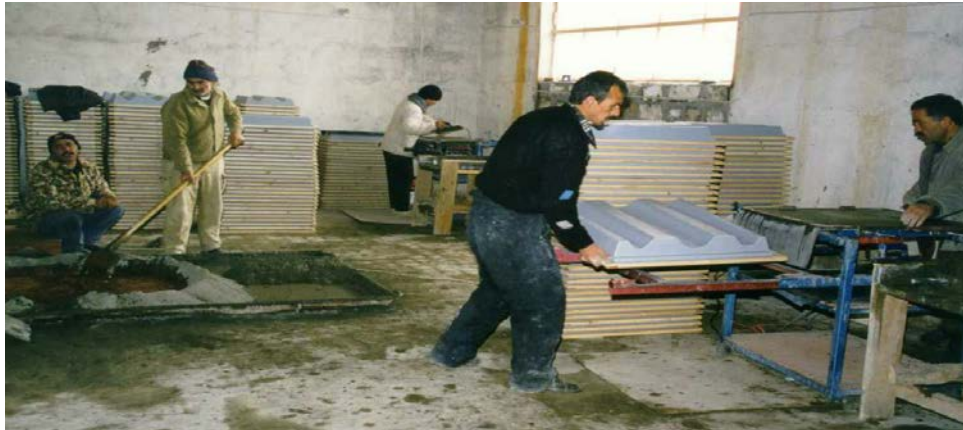
Figure 4.4 Mixing the mortar and assembling the table and mould
