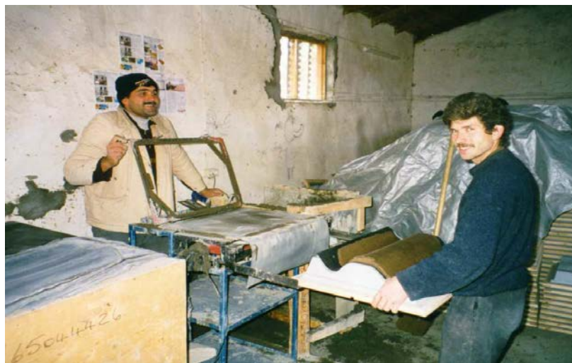
Figure 4.5 The frame is removed. The wet mortar is dragged onto the tile mould
