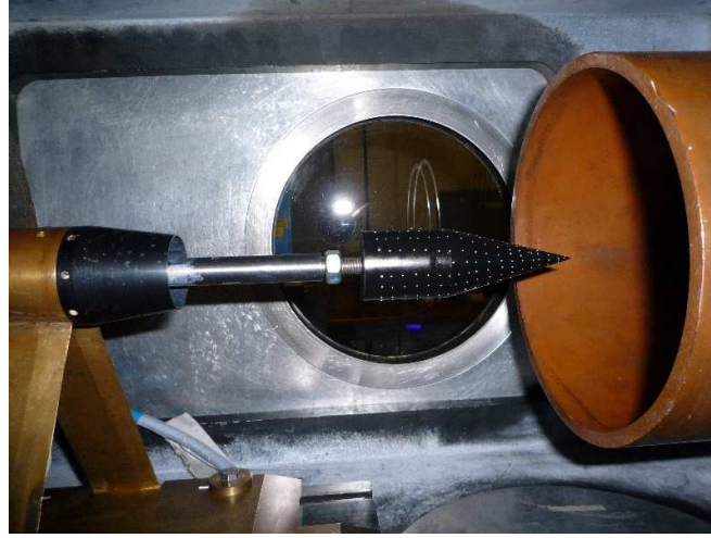
Figure 2.2: Test section of HSST with a cone-cylinder model placed on a sting.
