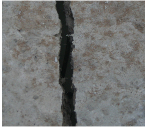
Figure 5-11 The fracture of the reinforcement with full -depth crack (G0F1)
