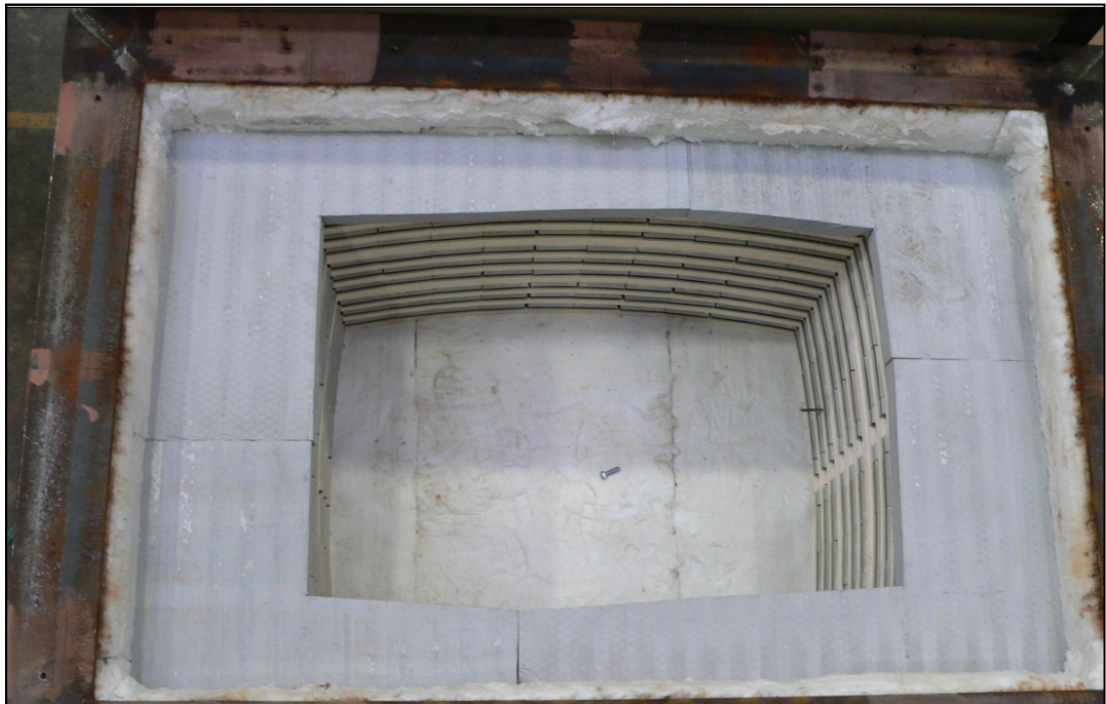
Figure 5-5 The electric kiln used to carry out the fire test
