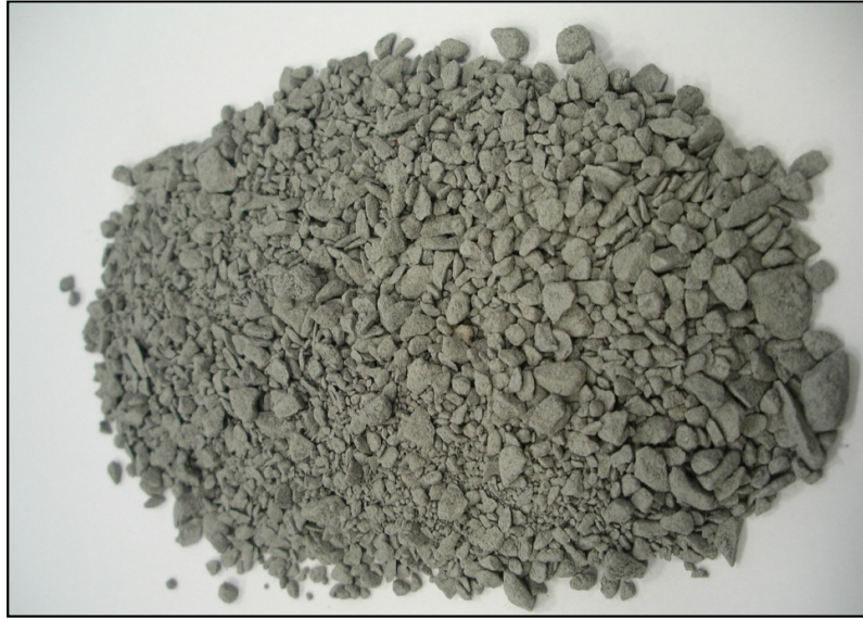
Figure 5-7. 6mm maximum size granular aggregate
