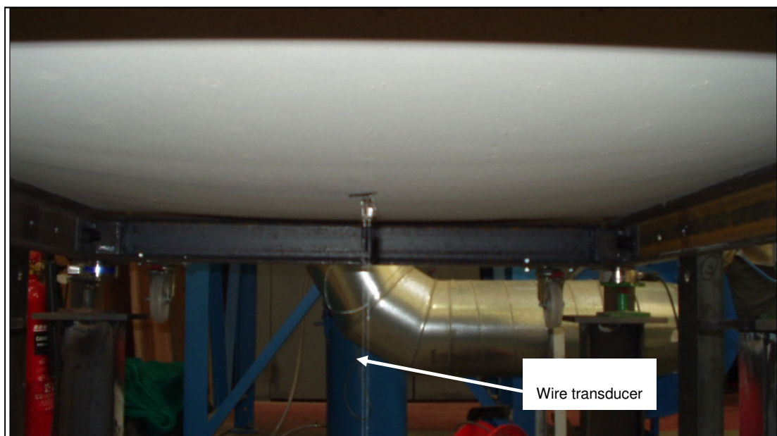
Figure 5-4 Wire displacement transducer
