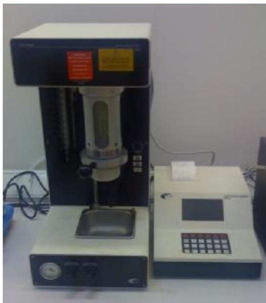
Figure I.5 HIAC ABS2 bottle sampler and HIAC 8000A liquid particle counter of particle size analyzer
