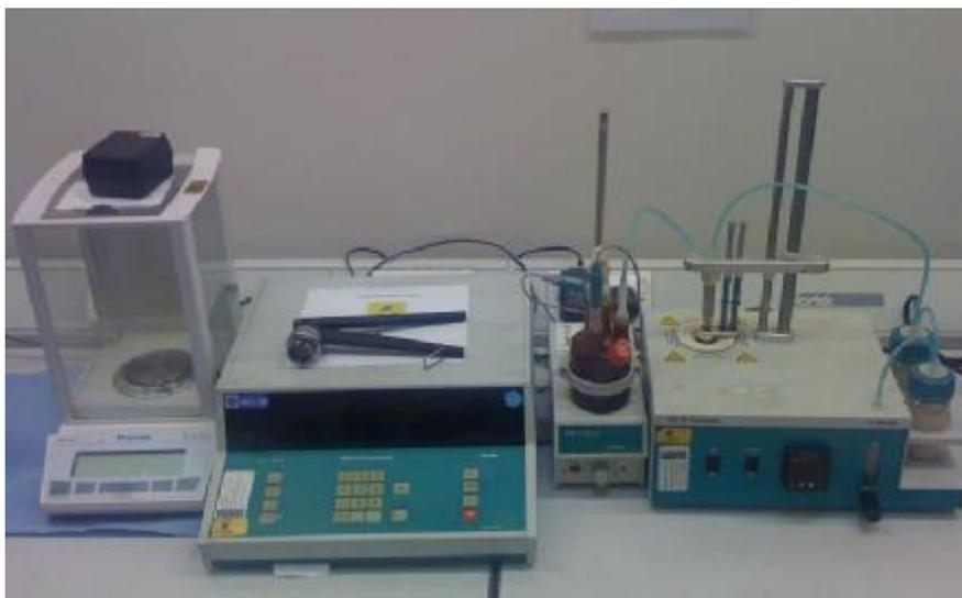
Figure I.4 The XB120 scale, 684 Coulometer and 832 Thermoprep of Karl Fischer titration equipment used for water content measurement
