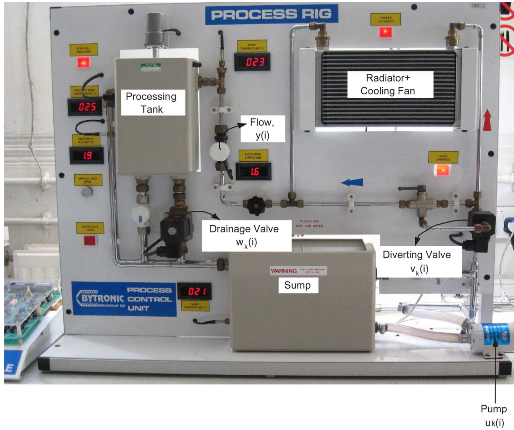
Fig. 3. Process control test rig at the University of Manchester.
