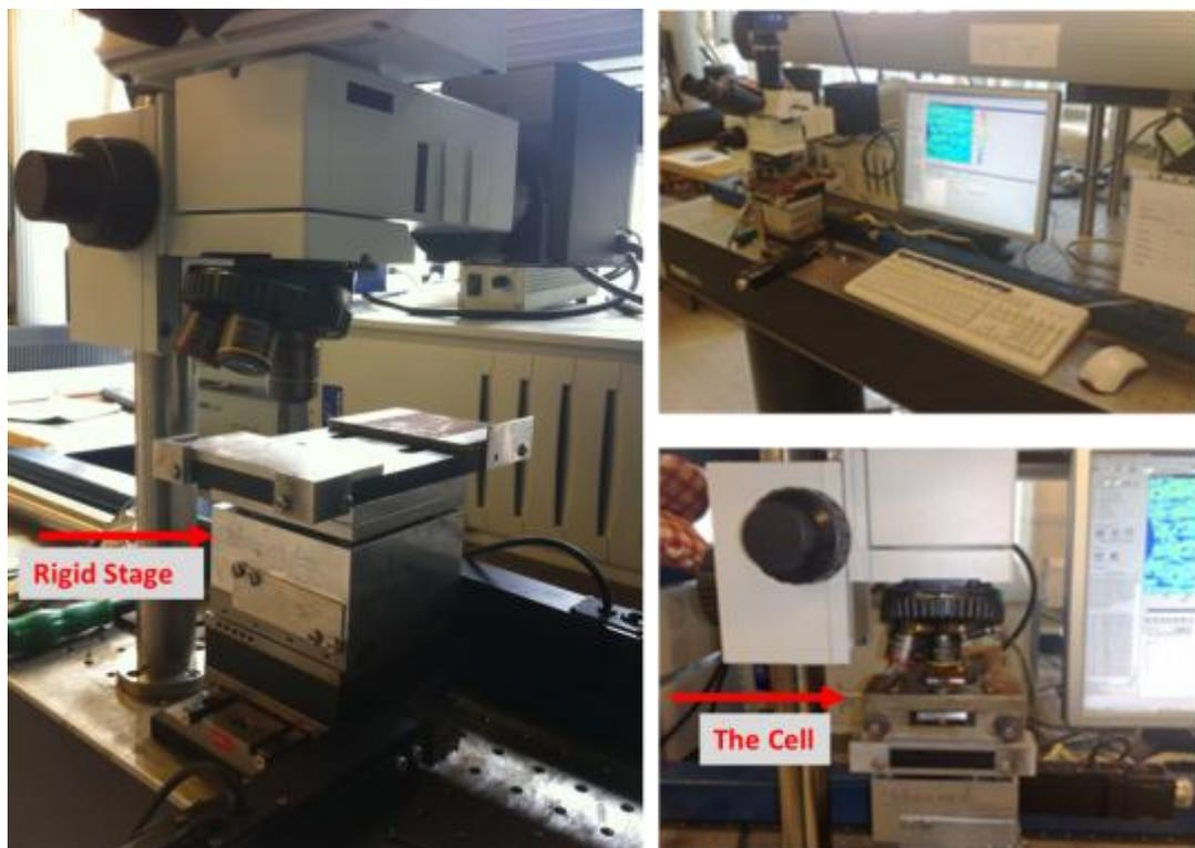
**Figure: 3-9: Setup of the rig under the DIC optical microscope.**
