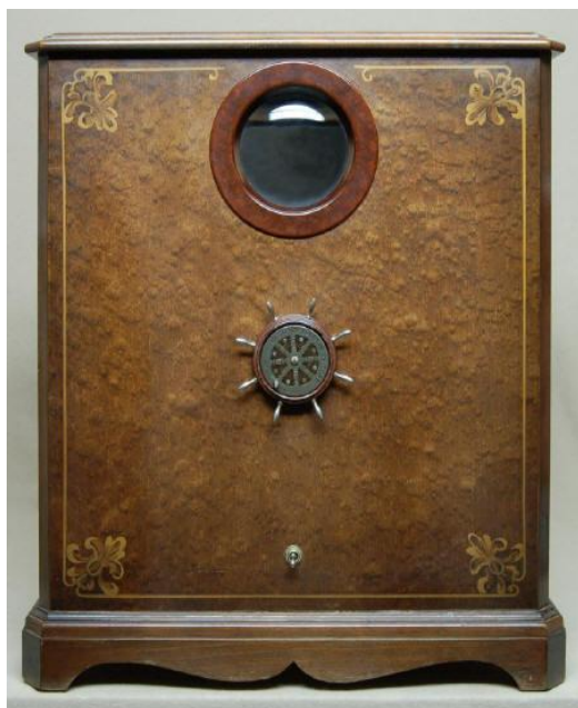
Figure 3.5a (top) Western Television Corp. contemporary advertisement for Western Television Visionette domestic television display, manufactured by Echophone Inc. Figure 3.5b (right) The tiny picture would be viewed through the 'porthole' with the other nautical reference, the ship's wheel, being used to adjust the picture phasing.
