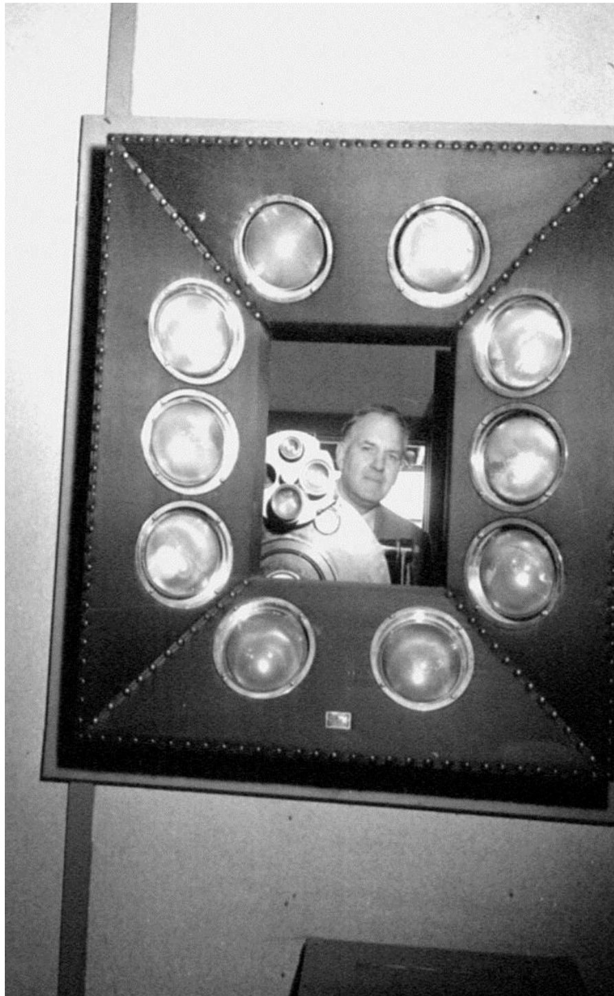
Figure 3.3 The performer's view of the television pick-up showing the bank of photo-cells in front with the Nipkow disc flying spot scanner behind and E B Kurtz of W9XK behind that. The performer would have been subjected to a very bright and rapidly moving probing spot of light.
