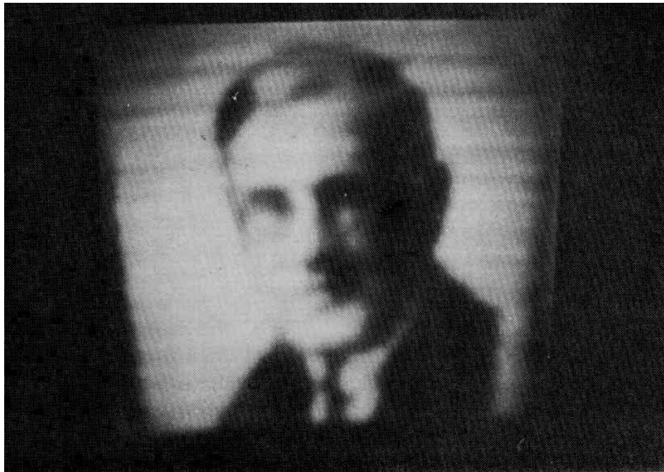
Figure 3.8 Off screen image from station W9XK television of a photograph of Walter A Jessup, former President of the State University of Iowa.
