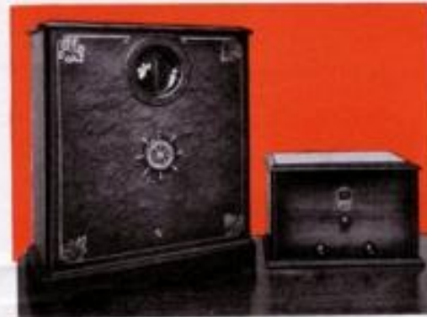
Complete Television Set. Visionette at left, Short Wave Receiver to the right.
