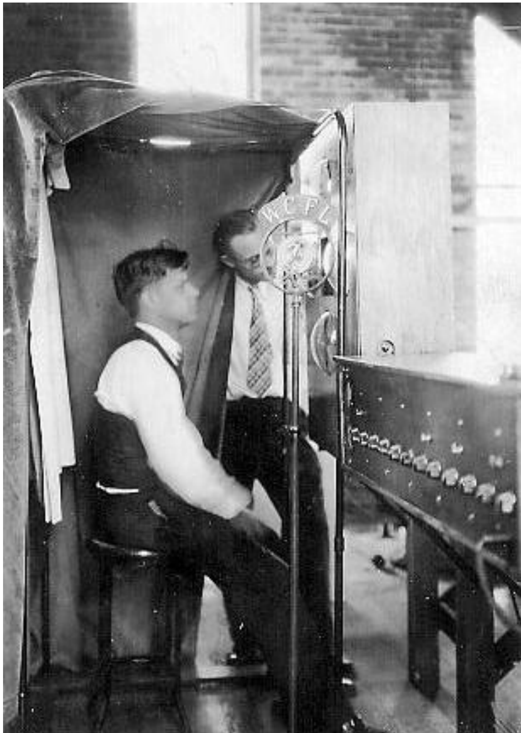
Figure 3.6 U A Sanabria seated in front of a flying spot scanner 1928
