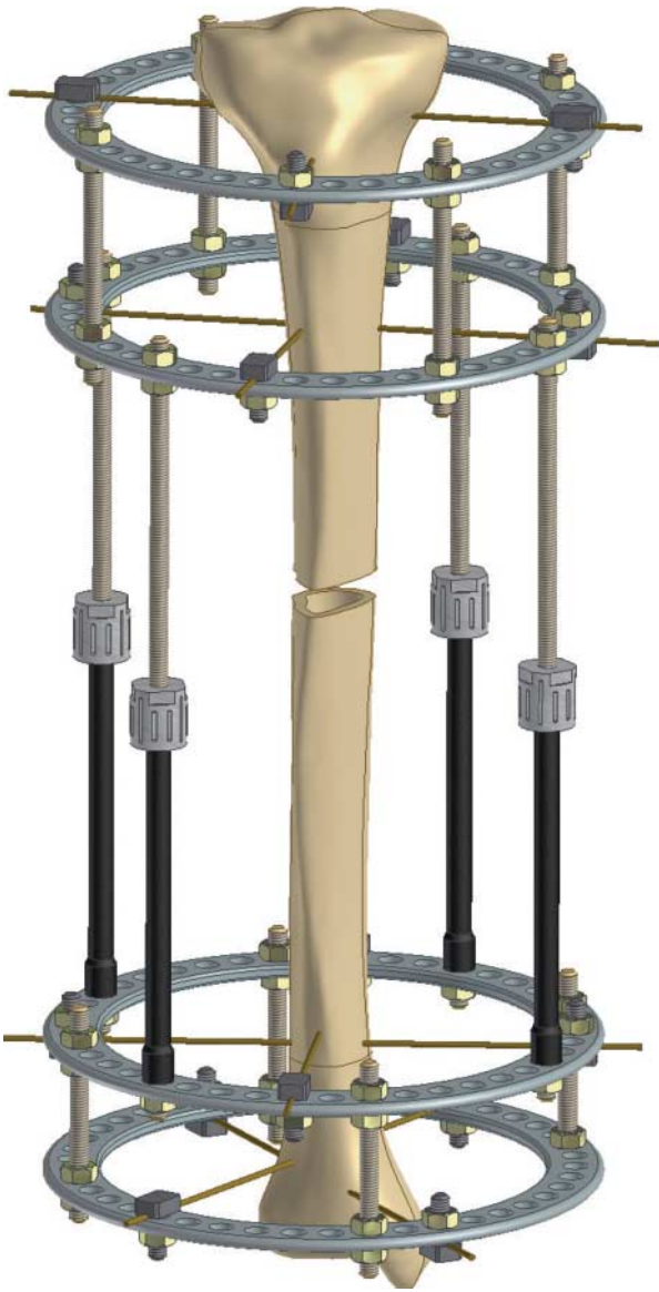
Figure 1. Full-ring Ilizarov frame applied for lengthening of tibia.
