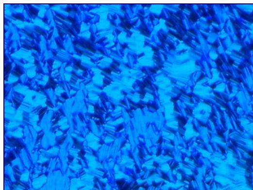
Figure 6.4 The optical fan-like texture of the hexagonal phase observed for 31% wt/ wt% Cu-phthalocyanine dye at 23.4°C temperature (magnification x ca. 200).
