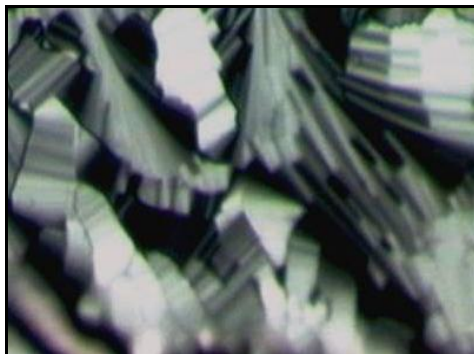
Figure 8.7 Mosaic texture appearing on heating the hexagonal sample of 26% wt/wt% black dye at 20°C (magnification \times ca.200).
