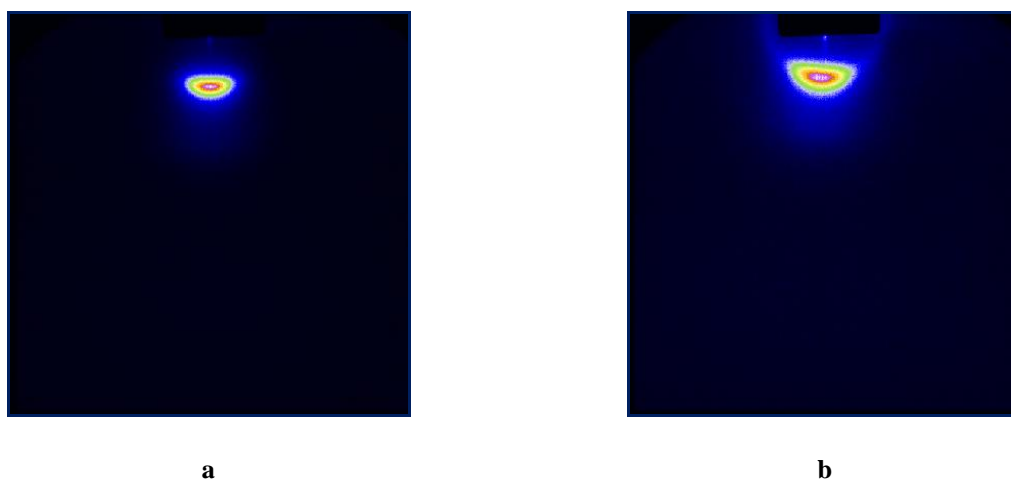
Figure 7.7 The small angle diffraction patterns of the nematic phase shown by Cu-phthalocyanine dye for 26% wt/wt% at 25°C (a) and 21% wt/wt% at 25°C (b).
