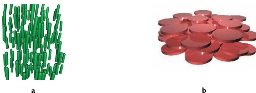
Figure 2.2 Main types of nematic liquid crystals: calamitics (a) [10], discotics (b) [11].
