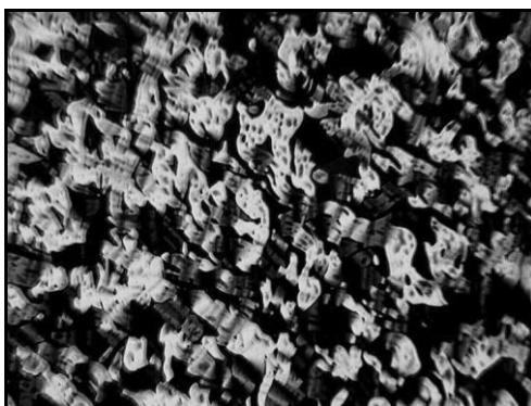
Figure 8.8 Melting of the nematic phase observed for 26% wt/wt% black dye at 57°C on heating (magnification \times ca. 100).
