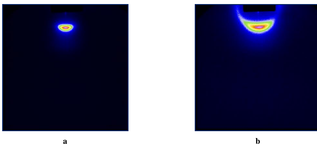
Figure 7.11 The small angle diffraction patterns of the nematic phase shown by Cu-phthalocyanine dye for 26% wt/wt% at 5°C (a) and 75°C (b).
