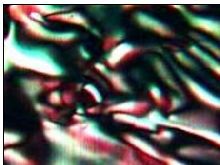
Figure 8.5 Nematic phase observed for 21% wt/wt% black dye at 21.8°C (magnification \times ca. 200).
