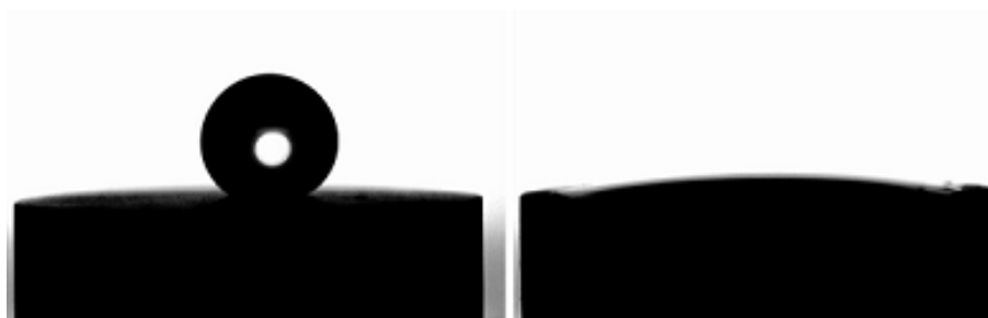
Figure 6.2: Water droplets on the surface of WE43 coated with sodium stearate (left and uncoated (right)).
