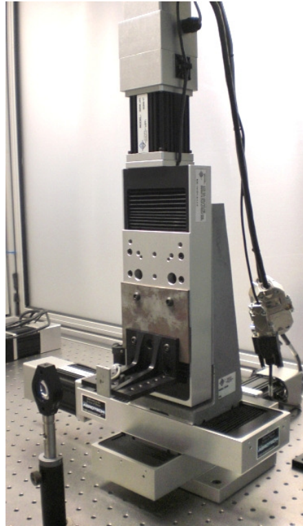
Figure 3.2 Three Axis Aerotech stage with focusing optics and target holder
