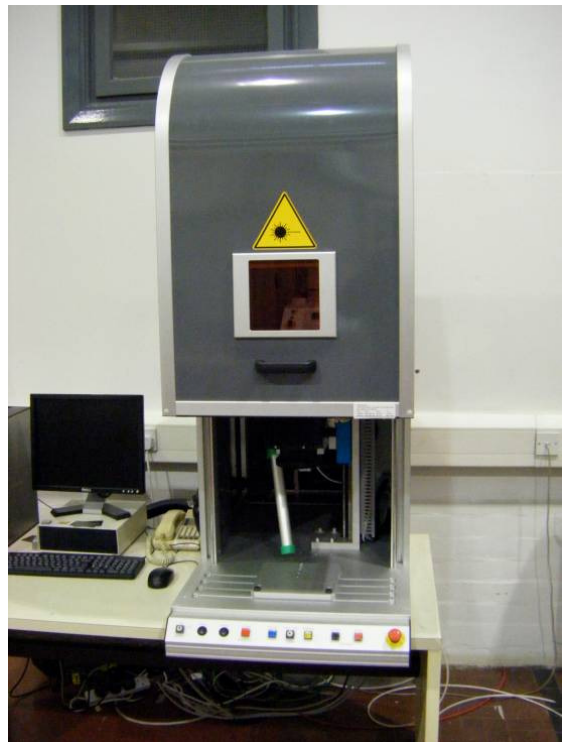
Figure 4.1 The enclosure which houses the Violino Marking System
