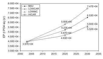
Fig. 8. Eutrophication potential (EP) for different scenarios.
