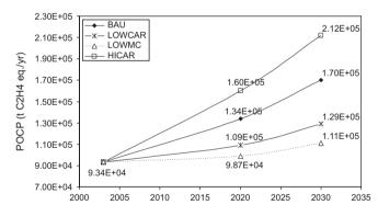
Fig. 6. Photochemical oxidation creation potential (POCP) for different scenarios.
