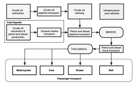
Fig. 2. The passenger transport system and system boundaries.
