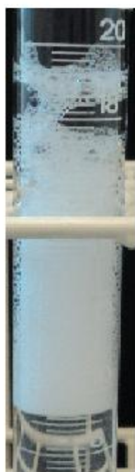
Fig 5.4.3. Top: 0.1 mg/ml 40K + (left to right) 0.1, 0.01, 0.001 mM SDS at 10 seconds after shaking. Middle: same samples after 5 minutes. Bottom left: 0.1 mg/ml 40K + 1 mM SDS at 10 seconds after shaking. Bottom right: 0.1 mg/ml 40K + 1 mM SDS after 5 minutes.
