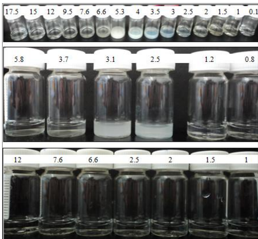
Fig. 6.1.3. Solutions of different concentrations of 40 KDa polypeptide with DTAB at concentrations as marked at the top of each bottle (in mM). (Top) 10 mg/ml of polypeptide. (Middle) 1 mg/ml of polypeptide. (Bottom) 0.3 mg/ml of polypeptide. All solutions were prepared at pH 5 and in 10 mM NaCl.
