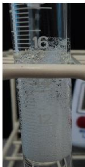
Fig 5.4.3. Top: 0.1 mg/ml 40K + (left to right) 0.1, 0.01, 0.001 mM SDS at 10 seconds after shaking. Middle: same samples after 5 minutes. Bottom left: 0.1 mg/ml 40K + 1 mM SDS at 10 seconds after shaking. Bottom right: 0.1 mg/ml 40K + 1 mM SDS after 5 minutes.
